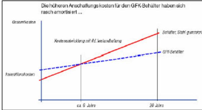
Above illustration compares investment costs/service costs of a rubber lined large diameter tank and GRP large diameter tank.
