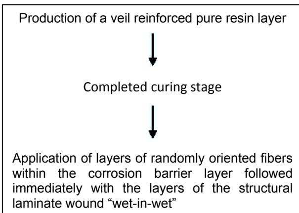
The laminates produced with this technique looked very good; however they increased the risk of blistering when put into practical use. The possible reasons for this were hinted at in section 1. The laminar boundary layer created between the hardened veil layer and the following layers is very thin and can be bypassed easily by diffusion. A balance is created between the flaking layer and the rim of the bubble, so that in the end many little blisters occurred.
