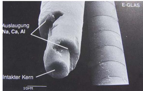
**Image 2.6: Damaged E-glass fibers after being stored in acid (REM-Image) [5]**
