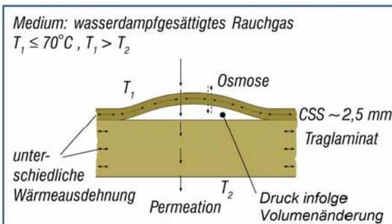
**Image. 2.5: Mechanism of blistering in FRP-parts [3]**
