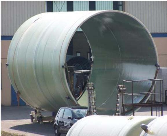
Image 6.1: Insulated 17'Ø flue gas duct section
