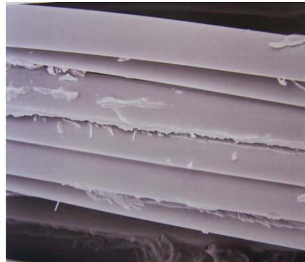
**Image 2.7: Intact E-CR-glass fibers from the inside of a blister (REM-Image) [4]**
